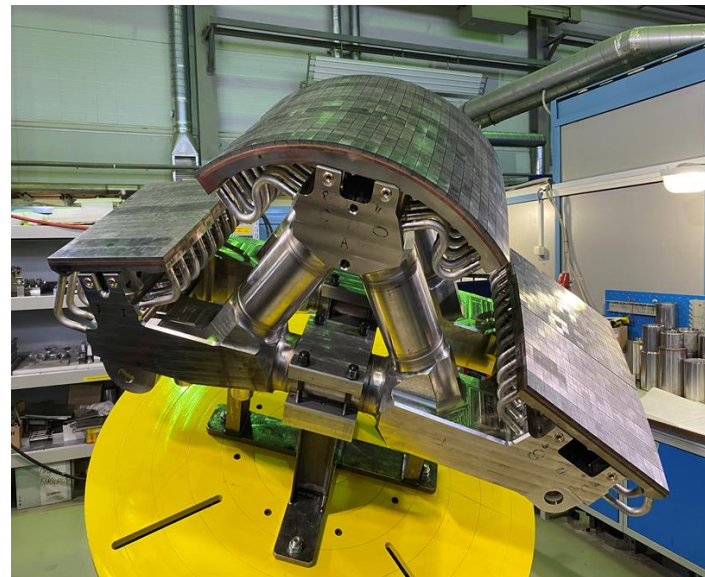
Full size prototype manufactured and supplied to ITER
