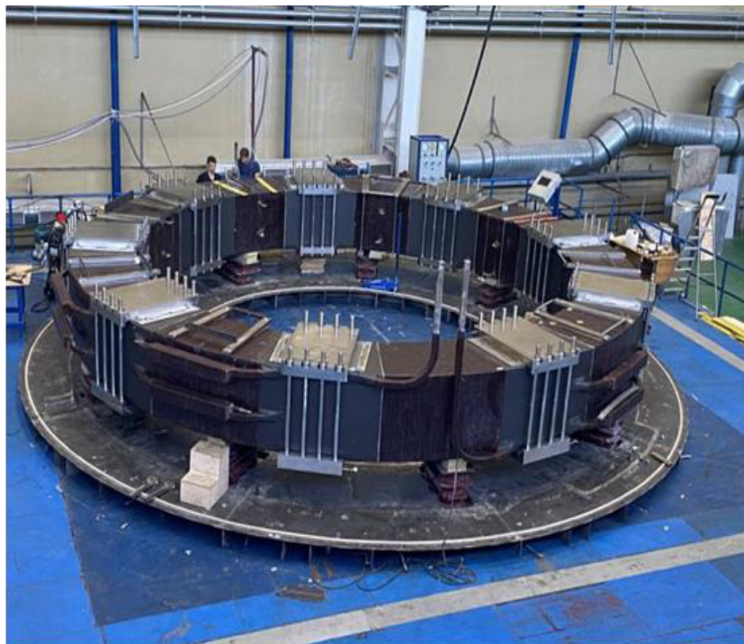
PF1 Magnet Coil with clamps installed
